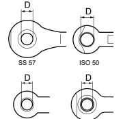
The wear limits for the bushing/wear ring in the drawbar eye are indicated in table.
